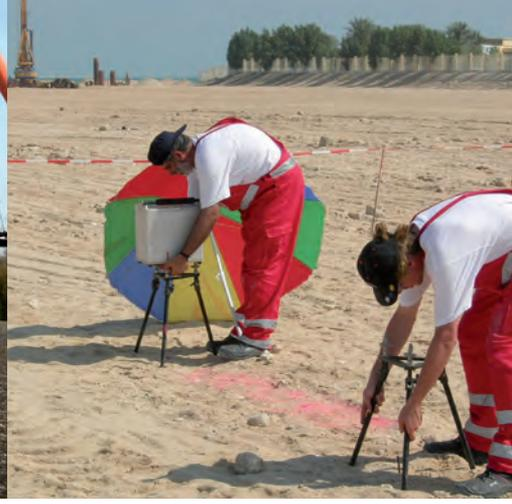
Gravity measurements during a construction site examination in Qatar
